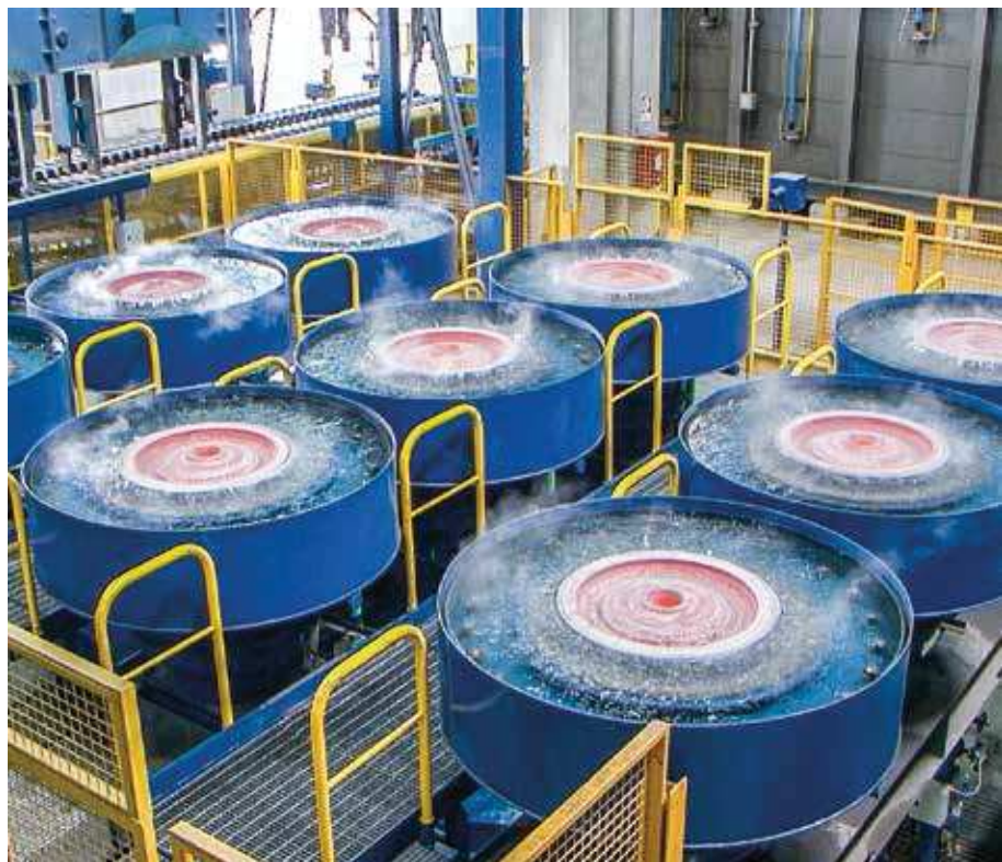
■ Differential Quenching System for Railway Wheels
