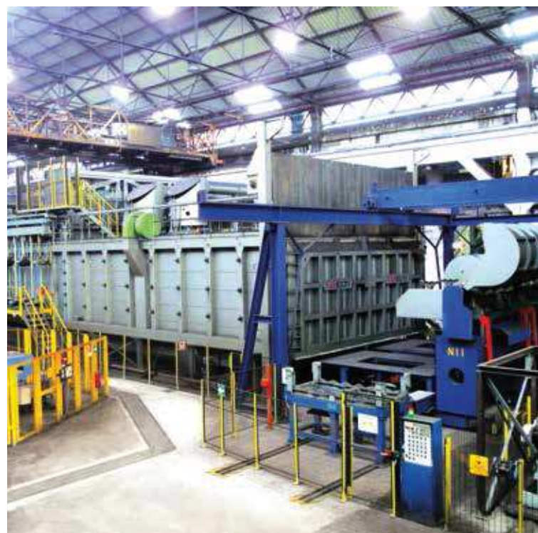
■ Walking Beam Heat Treatment Line for Railway Axles
