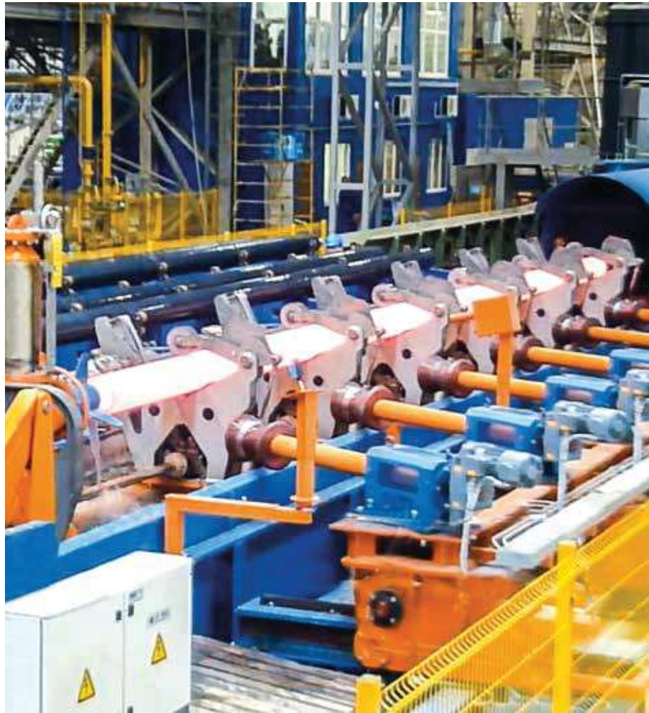
■ Quenching Tank System for Tubes
