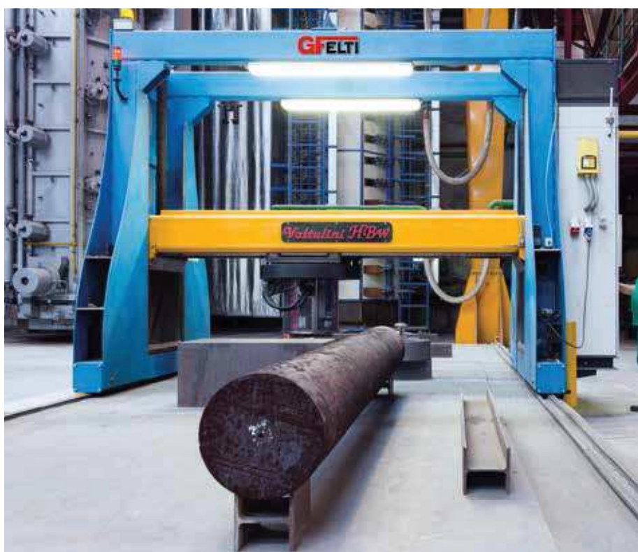
■ Automatic Plant with high productivity for Hardness Tests on Heat-Treated Products
