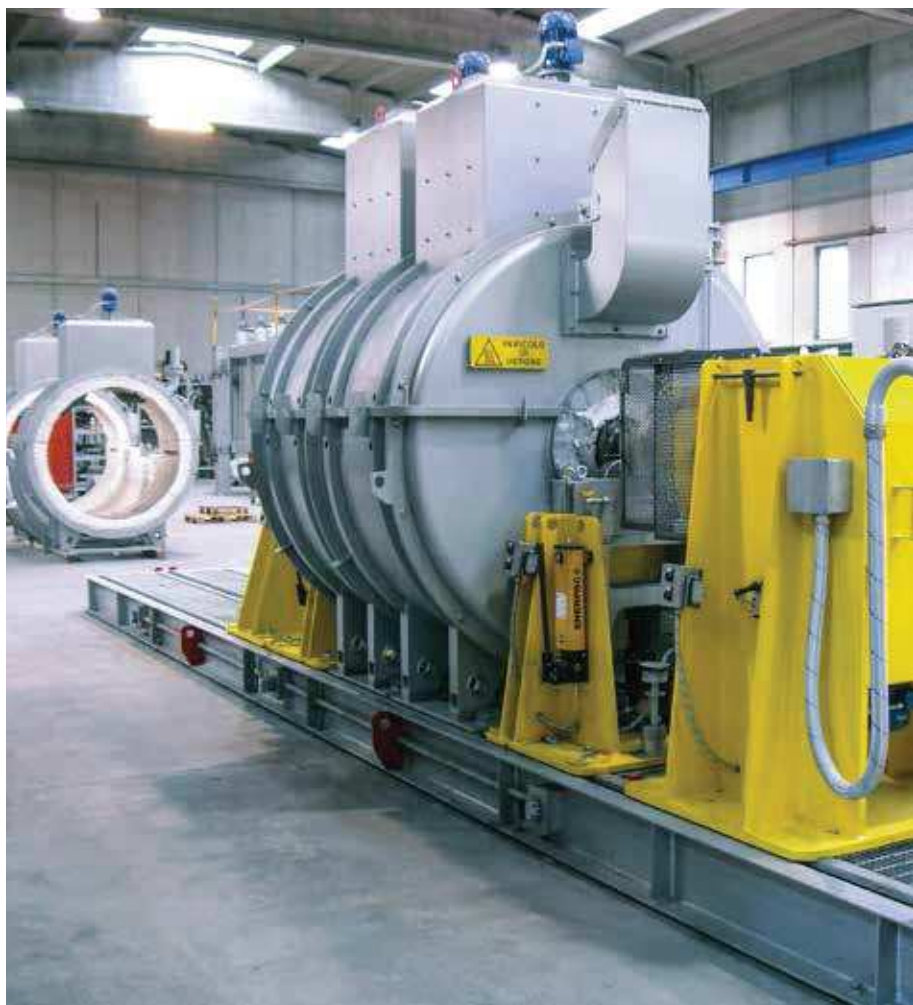
■ Equipment for Rotary Heat Stability Tests on Forged Rotors
